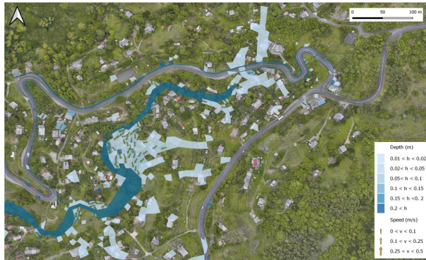
Flood mitigation Rodrigues - Quatre Vents, Dans Darisse - Current situation Velocity and Water depth - February 2019 rainfall event
